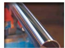
This shows a surface which has been pre-ground to Pyramid belt grade A6, P 2000. The surface is now silky smooth with a high sheen finish. With this finish we are now at the perfect stage to start polishing.
