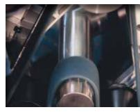
With a burnishing machine and a nylon web fleece belt you can remove minor scratches and achieve a smooth satin like finish in one easy step. Use on half speed, setting 3\*.
