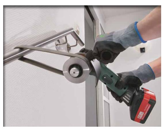
For closed off rail sections close to a wall the Metabo belt drum and "buttonhole" belt accessory option will prove particularly useful, especially if the rail is closed off with wall brackets on either side of your working area. With the buttonhole belts you can then loop & close the belt behind the rail. With this method you will achieve a perfect uniform result 3600 around the handrail. Going mobile? Go cordless with the S 18 LTX 115.
