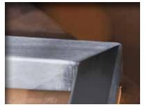
Remove the tape to reveal a perfectly finished mitre joint effect.
