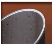
A pipe that has been deburred fully both inside and out.
