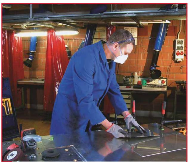
Use an aluminium or copper sheet as underlay for stainless steel sheets. This draws off the heat when working helping to prevent the sheet from warping. In addition an underlay will prevent any possible contact corrosion with ferrous metals, e.g. an iron welding table.
