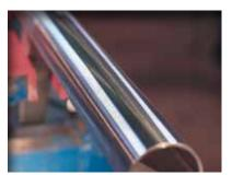
Minor structural grooves on the pipe.
