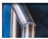
TIG welding seam on a handrail corner.
