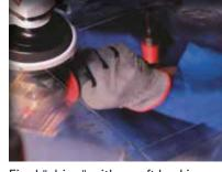
Final "shine" with a soft backing pad and a soft cling-fit fleece disc in combination with blue polishing paste at speed setting 4-5\*. Start off slow, work the paste into the material and finish on high speed.
