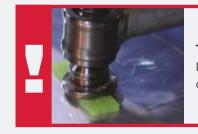
Protect your surfaces from scratches using plastic mats when clamping.
