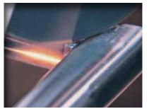
The KNS fillet weld grinder is the machine of choice for this task thanks to its ultra slim profile. Select speed setting 5\* and remove the fillet weld seam easily, even right into the corner without damaging neighbouring surfaces.
