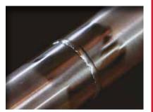
Slightly rounded welding seam, the tarnish has been removed.
