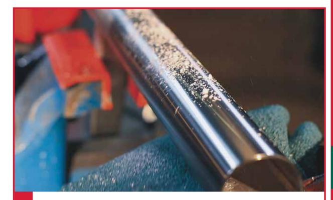
Remove any polishing paste residue evenly and gently from stainless steel surfaces using talc (6.26399) and a micro-fibre cloth (6.26398).
