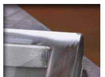
After the weld seam has been removed burnish one side of the box section using the P 60 wheel in a linear motion. If so required be careful to not round the edges.
