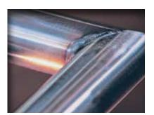
Right angle weld seam on a handrail.
