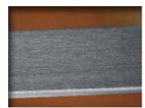
A longitudinal grinding pattern, the rolled skin has been removed completely.
