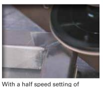
around 3\* you can use the hard backing pad with the Pyramid sanding media to remove the weld seam. Select the grit of your choice. A 45 or A 30 grit could be used here. By using the hard backing pad option instead of the soft and flexible KLS disc your edges will stay intact, thus helping to avoid any 'rounding off'.
