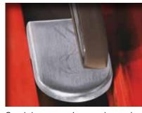
Sand the area using a nylon web fleece band on full speed with the grinding belt arm 6.26381 which has a 13 mm wide support pad.
