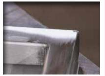
Weld seam removed. Turn to the next page for further steps.
